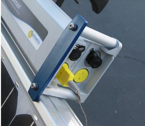
**Figure 16. Thermocouple plugged into the TC1 connector.**
