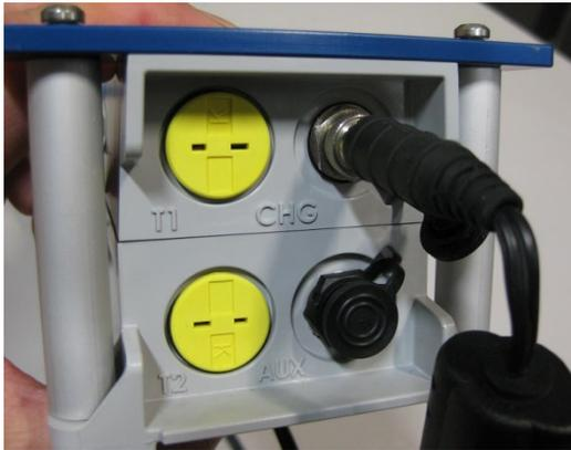
**Figure 9. Charger connected**
