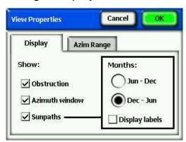
In the Display tab, select what data will be displayed on the graph: Obstruction is the elevation data with one degree resolution; Azimuth window is the section of azimuth values for which the maximum (or average) data will be displayed; and Sunpaths. Also select which month labels will be displayed on the sunpaths, Jun-Dec or Dec-Jun.
