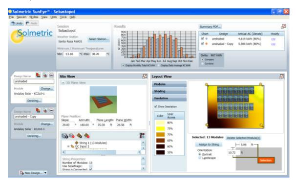
Figure 8. Solmetric PV Designer software screen.
