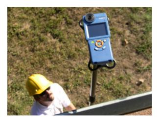
Figure 7. SunEye Extension Kit enables measurements up to 18 feet above ground level.
