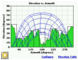
Figure 4: Obstruction Elevation view
