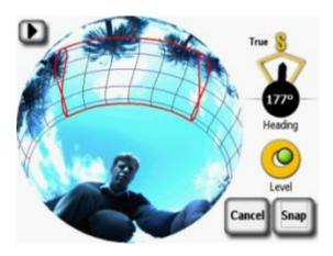
Figure 5.. Identify shade-free areas using SunEye window.
