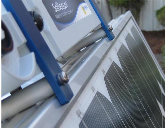
**Figure 19. SolSensor correctly seated along the upper horizontal leg of the module frame.**
