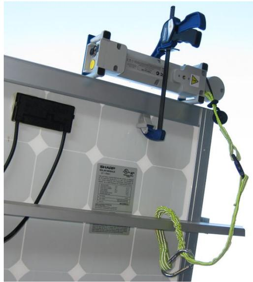
**Figure 18. SolSensor tool lanyard secured to a racking member.**
