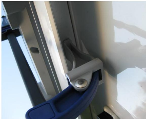
**Figure 20. Tip of frame clamp properly seated on inside surface of module frame**
