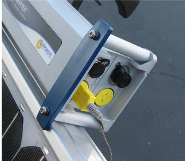
**Figure 21. Thermocouple plugged into the TC1 connector.**
