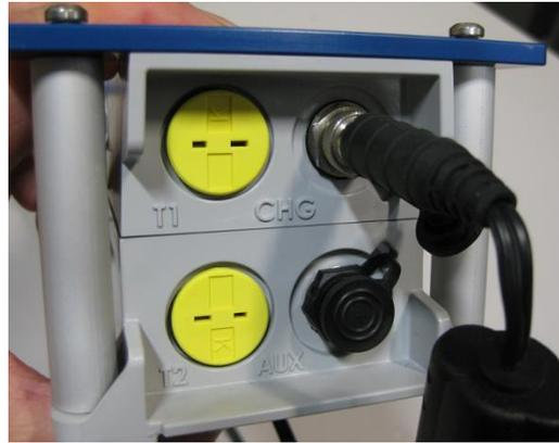
**Figure 13. Charger connected**
