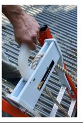
**Warning:** Do not operate the Module Lift in windy conditions or the module may be lifted off the ladder causing property damage, injury, or death.
