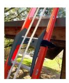
*Warning:* Ramp must be positioned so that when a module slides up the rails of the ladder, it will not make contact with a ladder strap.
